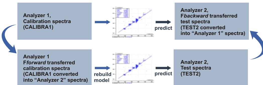
**Figure 2.** Top: Backward calibration transfer: TEST2 data from Analyzer 2 are adjusted so that they can be predicted with the model built on the CALIBRA1 data from Analyzer 1. Bottom: Forward calibration transfer: CALIBRA1 data from Analyzer 1 are first transformed so that their calibration model can predict the TEST2 data from Analyzer 2 directly.
