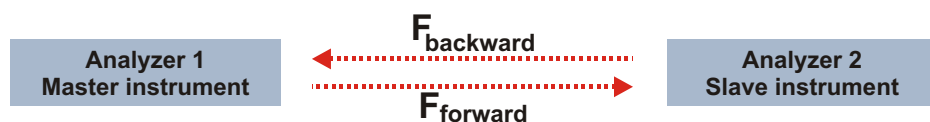
Figure 1. Scheme of backward and forward methods of calibration transfer. A calibration is developed on a master instrument (Analyzer 1), while predictions will occur on spectra from a slave instrument (Analyzer 2). F_{backward} and F_{forward} are the transfer matrices for each direction respectively.
